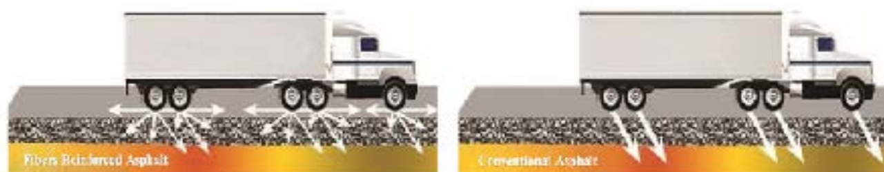
Fig. 1: The performance of the fibers in Asphalt Concrete (4)
